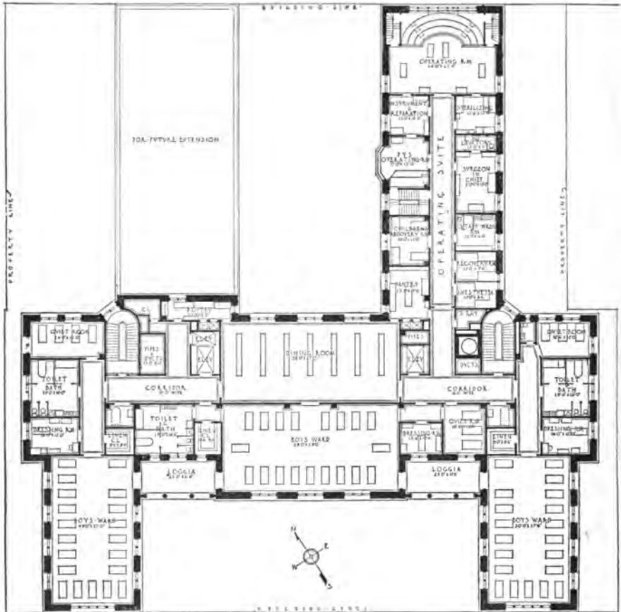
NEW YORK HOSPITAL FOR THE RUPTURED AND CRIPPLED Fourth Floor Plan
